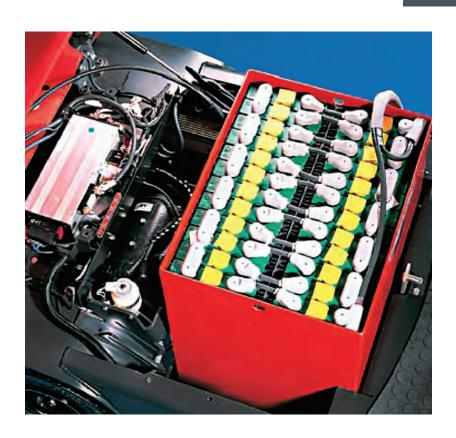
The advanced, energy efficient digital controller provides infinitely smooth acceleration and traction for safe, efficient towing duties. The driver is always in control even on a gradient where automatic regenerative braking occurs as the accelerator pedal is released, ensuring that the tractor descends the gradient at a controlled rate thus preventing overspeeding.
