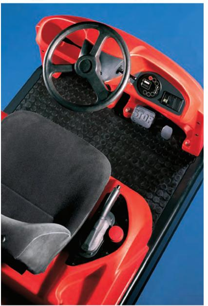
Comprehensive instrumentation displays a continuous status report indicating elapsed time, battery state of charge, brush wear, low brake fluid level and motor over temperature thus allowing charging schedules and routine maintenance to be carried out at optimum intervals, resulting in increased uptime and maximum productivity with lower operating costs.
