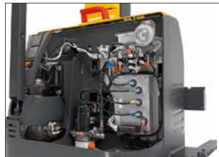
Sealed AC motor, controllers and connectors
